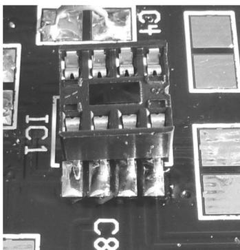
Tin the pads for IC1 and IC2.
