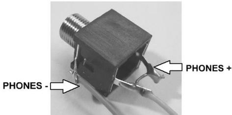
To enable a pair of “walkman-type” headphones to be used with the receiver the phones socket must be connected as shown. The two connectors at the back of the socket are joined and connected to the **PHONES +** pad and the connector at the front is connected to the **PHONES -** pad. We suggest that you connect the wires to the socket first, cut them to length (3 to 4cm) and then solder the other ends to the board before fixing the socket to the front panel as space is a little tight here.
