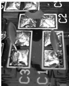
The capacitors (C1 to C18) can now be mounted; trimming and bending the leads for soldering to the pads. The value designation for each capacitor is shown in the parts list. Check carefully that the correct capacitor is chosen for each place.
