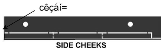
Adding the side cheeks at this point does mean that the fixing of the front and back panels of the receiver is much easier. Attaching the side cheeks does require a really hot soldering iron bit and plenty of solder. We suggest that you begin with a large blob of solder at each end to fix the position. Attempt to get the side cheek as near vertical as possible. You may freely run more solder along the narrow pads on the length of the board.
