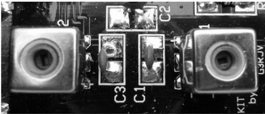
The two input tuned circuits L1/C1 and L2/C3 are set to maximum output using the cores in L1 and L2. Use a trimming tool or work very carefully with a small slotted screwdriver. L1 and L2 can be peaked for maximum signal strength using a signal generator or amateur
