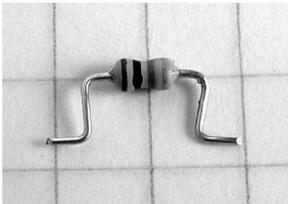
The passive components (resistors and capacitors) can now be added. Begin with the resistors (R1 to R6). The colour code for the resistors is given in the parts list. To enable a secure solder connection of the parts, the leads are bent into an “L” shape for adding to the pads on the board.
