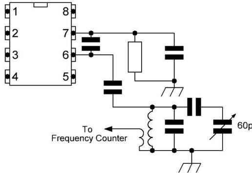
L3, the oscillator coil, has an unused link winding. This may be used to feed a frequency counter. Connect one (either) side of the link winding to ground and use the other end to connect to the counter. Some counters may detune the frequency a little so putting a low value capacitor (10 to 22pF) between the counter and the link winding is advised. Set the Tuning Capacitor control fully anti-clockwise and adjust the core to read
