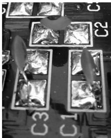
The capacitors (C1 to C18) can now be mounted; trimming and bending the leads for soldering to the pads. The value designation for each capacitor is shown in the parts list. Check carefully that the correct capacitor is chosen for each place. Note that C11 is not used on the 160m version of the kit.
