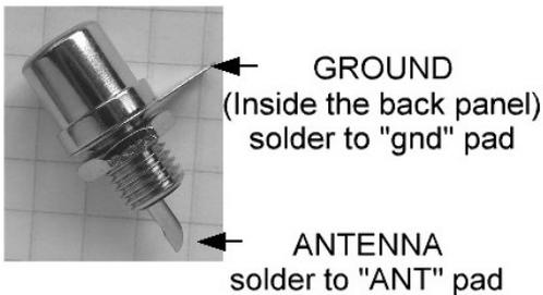
The antenna input socket is a single hole fixing ‘phono socket’. It has a ground connection tag that needs to be inside the back panel. Bend this tag inwards for a wire that connects to the “gnd” pad. The antenna input connection is soldered to the “ANT” pad. Use differing colours to identify the two leads and twist them together.
