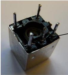
The oscillator coil, L3, is a 45u0L component, and the bandpass filter coils, L1 and L2, are also 45u0L components.
