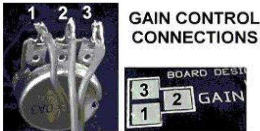
The gain potentiometer connections are shown; numbered 1, 2 and 3.
