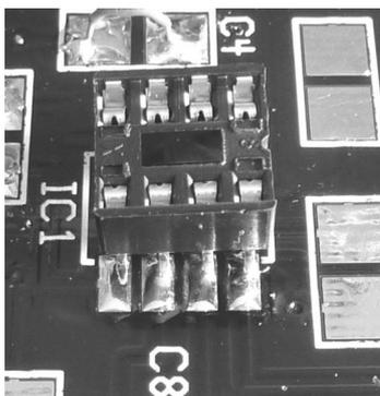
Tin the pads for IC1 and IC2.
