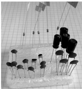
There is merit in following this order in construction. Note that the instructions refer to having the board so that the legends for the components read the correct way round (PP3 at the top right). The best results will come from the use of medium size soldering iron and Tin/Lead solder. It does help to set out all the components in the order they will be used. The best way is to use a small piece of polystyrene to hold the individual parts.
