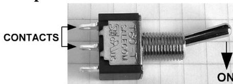
The power switch enables the PP3 battery to be switched on and off. When the switch level is in the down position, the two contacts marked here will be joined. Use two wires to connect these contacts to the **SW** pads (either way round).
