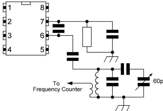
L3, the oscillator coil, has an unused link winding. This may be used to feed a frequency counter. Connect one (either) side of the link winding to ground and use the other end to connect to the counter. Some counters may detune the frequency a little so putting a low value capacitor (47 to 100pF) between the counter and the link winding is advised. Set the Tuning Capacitor control fully anti-clockwise and adjust the core to
