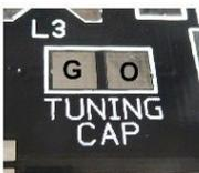
The connections to the pads on the board are shown here. The capacitor should be mounted tags downwards — this makes the connections shorter. If you get the connections reversed, the receiver will still work, but there will be a change of frequency as your hand approaches the tuning control.
