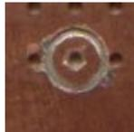
This method can give the constructor complete freedom of layout. You can cut a few pads, mount some components, and then cut a few more. The tool can simply be twisted by hand - just cover the shank with tape to avoid cut fingers.
