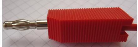
terminated with crocodile clips and the red and black leads are terminated with 4mm plugs (the standard plug used in test meters). If your meter uses a different size of plug, then you will have to obtain these yourself. The placement of the four leads is shown in the circuit drawing. Later the diode probe will be converted into a basic wameter to measure the final transmier output.
