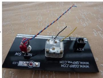
Now remove the insulation completely from two 2cm pieces of the black wire, and solder one end of each piece of bare wire to the KEY pads on the main board. Be careful you don't catch your fingers on these when they are stuck up in the air!
