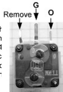
The tuning capacitor is mounted to the front panel using the two small screws provided. It is mounted tags downward.
