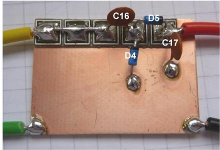
Tes5ng the transmier at this stage requires a Diode Probe. All the parts are provided for making such a probe as shown in the picture.
