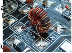
The transmitter is built in two sections; the first being the oscillator section. This includes the OSCILLATOR, the DRIVER and the KEY SWITCH. These are then tested before the rest of the stages are added.
