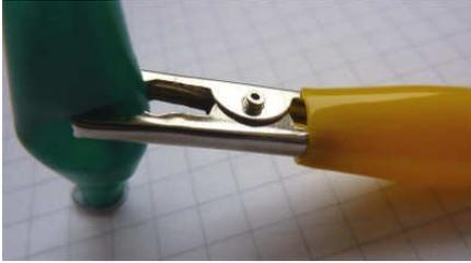
The clip is chromium plated and soldering will be much easier if the area to take the solder is roughed a little with emery paper or the
