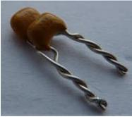
Nearly all the capacitors in the filter are actually two in parallel as the correct values are not commercially available. We suggest that you parallel these pairs first as shown here, before fiGng them. A good plan is to mount C12 - C15, and C18, then mount L5, followed by L4 and L6.
