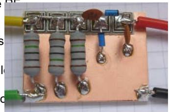
Connect the yellow clip lead to the centre of the ANT socket and the green clip to the ground of the ANT socket and the red and black leads to a voltmeter. Connect the 12 volt supply, leaving the NET SW switch upwards, and press the Morse KEY down. Read the output voltage. The
