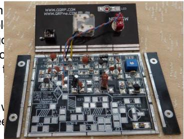
This picture shows that done, and the correct vertical position of the side panels although they have not been soldered into place yet.
