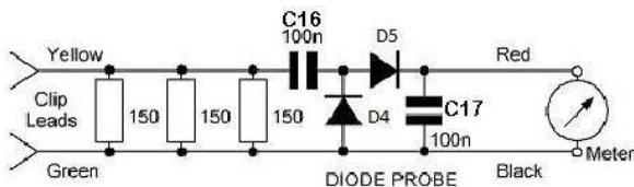
voltage is the peak to peak measurement. If you are going to use the RF wameter o6en, then we suggest that you replace the yellow and green leads with a shor4sh piece of 50 Ohm coax terminated in a Phono (RCA)plug. The inner
