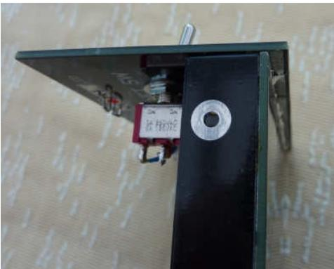
Like the side cheeks the front panel is soldered to the main board. This panel, unlike the side cheeks, overlaps the base board. The base board should be put in the gap between the soldered tracks at the bottom of the front panel. This picture shows the correct position of the front panel against the base. Again, we suggest that you use the “one blob” technique underneath the board to get the panel aligned correctly and vertical. Add a second blob when you are happy with the alignment,
