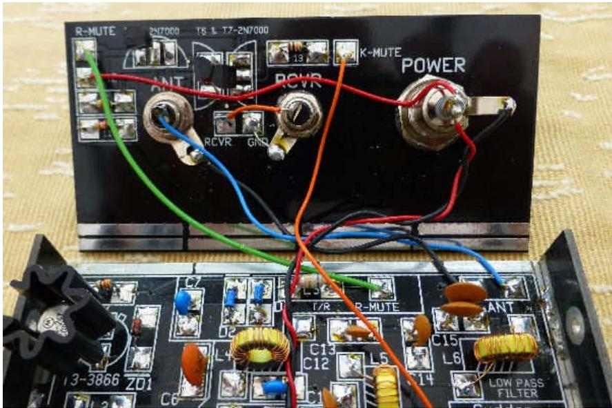
Finally, having finished the wiring to the back panel, you should solder the back panel in place using the same method that you used for the front panel. Be careful when soldering near the wires as the insulation is easily damaged by the soldering iron. There is enough length to move them out of the way of the iron.
