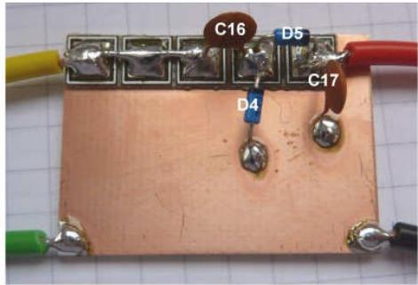
Tes4ng the transmier at this stage requires a Diode Probe. All the pa are provided for making such a probe : shown in the picture.
