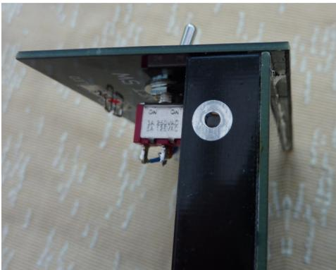
Like the side cheeks the front panel is soldered to the main board. This panel, unlike the side cheeks, overlaps the base board. The base board should be put in the gap between the soldered tracks at the boom of the front panel. This picture shows the correct posi2on of the front panel against the base. Again, we suggest that you use the “one blob” technique underneath the board to get the panel aligned correctly and ver2cal. Add a second blob when you are happy with the alignment,
