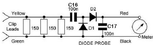
voltage is the peak to peak measurement. If you are going to use the RF wattmeter often, then we suggest that you replace the yellow and green leads with a short piece of 50 Ohm coax terminated in a Phono (RCA) plug. The inner conductor should go where the yellow
