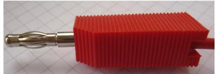
(the standard plug used in test meters). If your meter uses a different size of plug, then you will have to obtain these yourself. The placement of the four leads is shown in the circuit drawing. Later the diode probe will be converted into a basic wattmeter to measure the final transformer output.
