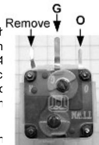
The tuning capacitor is mounted to the front panel using the small screws provided. It is mounted tags downward.
