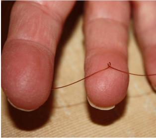
Sometimes if the wire gets twisted and forms a loop it results in a kink. Untwist the wire carefully. Trying to pull out the kink can snap the wire. Complete the 25 turns. They should occupy about three-quarters of the circumference. The 5 turn link winding, using red wire, is added over the centre of the main winding. Guess the centre, it is not really critical
