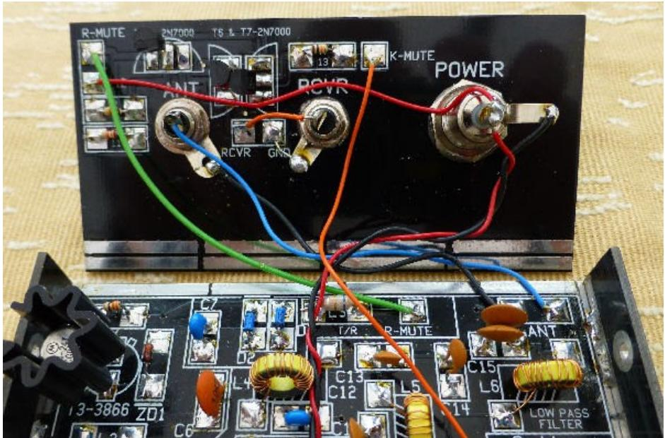
Finally, having finished the wiring to the back panel, you should solder the back panel in place using the same method that you used for the front panel. Be careful when soldering near the wires as the insula2on is easily damaged by the soldering iron. There is enough length to move them out of the way of the iron.
