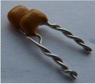
Some of the capacitors in the filter are actually two in parallel as the correct values are not commercially available. We suggest that you parallel these pairs first as shown here, before fitting them. A good plan is to mount C12 - C15, and C18, then mount L5, followed by L4 and L6.
