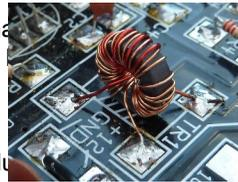
The transmitter is built in two sections; the first being the oscillator section. This includes the OSCILLATOR, the DRIVER and the KEY SWITCH. These are then tested before the rest of the stages are added.
