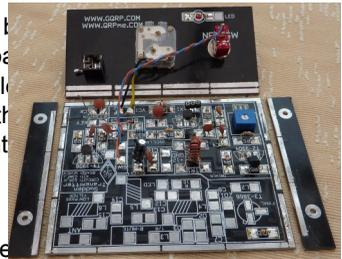
This picture shows that done, and the correct way round of the side panels although they have not been soldered into place yet.
