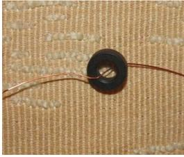
Winding toroidal coils is easy. It just requires patience and care. TR1 uses the black core with the gold wire for the main winding. The 25 turns require 15" of wire. Each time the wire passes through the hole (including the first time) it counts as ONE turn. Hold the core firmly with one hand and
