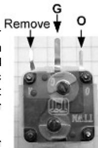
The tuning capacitor is mounted to the front panel using the small screws provided. It is mounted face downward.
