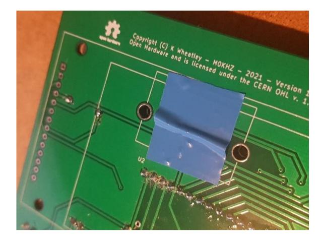
This is merely a safety precaution as a metal cover on the back of the display ends up quite close to these pins.
