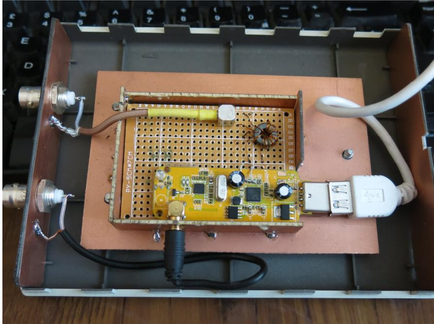
You can see above that the original VHF/UHF connection to the dongle has been preserved and you simply need to switch the SDR software settings when you want to use the HF port. The dongle's USB connection was extended using a cable.
