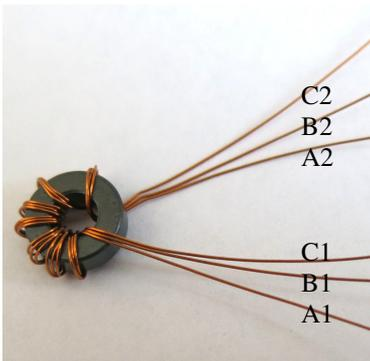
C1 & B2 Join together and insulate.
