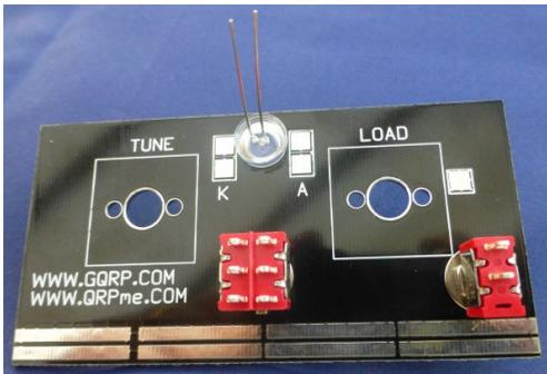
panel, the shorter lead is the cathode and is on the TUNE control side. Note the way up of the switch S2.
