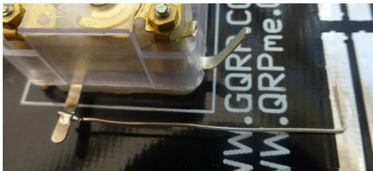
Next, using a short length of BT wire, connect the two bottom tags of the LOAD capacitor together and to the lower tag of S2, then connect the 470pF capacitor between the upper tag of S2 and the side tag of the LOAD capacitor. For all these connections to the capacitor, make a small hook at the end of the wire, and squeeze it up to gently grip the capacitor tag.
