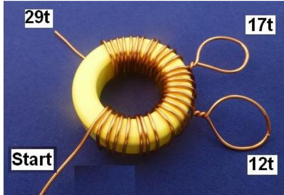
The Primary winding (shown above) has 29 turns of 20swg wire (the thickest wire), tapped at 12 turns and 17 turns. This requires about 50 inches of wire. Each pass of the wire
