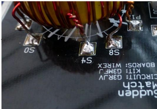
Finally for this stage of the construction, solder in the rest of the parts on the main board. It would be better not to overheat the diode and make sure that you get it the right way round - both the diode and the board legend have polarity bars at the end. The resistors should be mounted, like the coil, by making a foot on the end of the wire thus having the resistors some 10mm above the board. This also applies to the ceramic capacitor.
