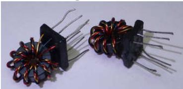
Trifilar transformers by Ashar Farhan – limited quantity. The toroid is probably FT37 size and the wire is approx. 26SWG. 50p each max of 4.
