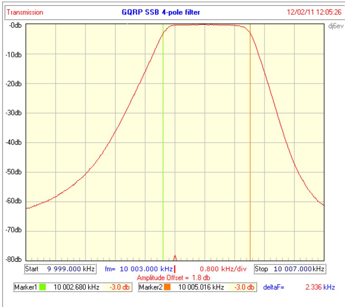
**Fig 3** This is the frequency response of the 4-pole filter. I would regard this as the minimum performance for either a transmitter, or a receiver. For this reason the club is selling the crystals in batches of ten. This number will allow the selection of sufficiently well-matched crystals for at least a 6-pole filter.
