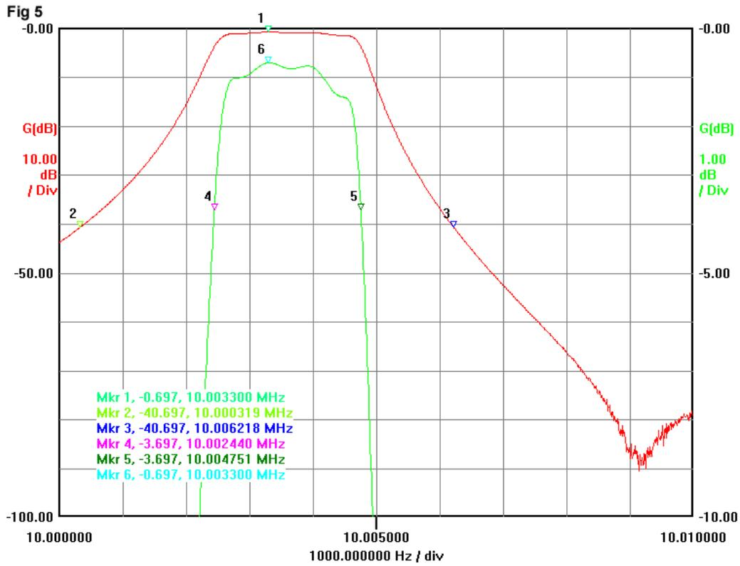
Fig 5 This is a detailed view of the pass-band and the stop-band. Here you can see the depth of the notch caused by the parallel resonance of the crystals. It will be even deeper in higher-order filters but will be hidden by the circuit noise.
