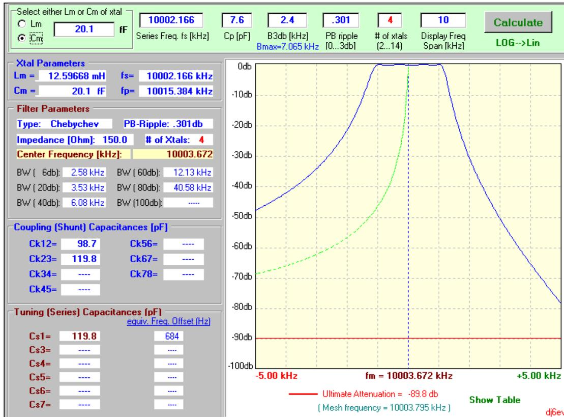
**Fig 1a** shows a screen shot of the Dishal program which was written by Horst Steder DJ6EV. The input parameters are entered in the seven boxes in the top panel. Pressing the ‘Calculate’ button displays the component values on the left-hand side of the display. A graphical display of the frequency response is shown on the right-hand side, also.
