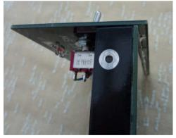
Like the side cheeks the front panel is soldered to the main board. This panel, unlike the side cheeks, overlaps the base board. The base board should be put in the gap between the soldered tracks at the boom of the front panel. This picture shows the correct posi4on of the front panel against the base. Again, we suggest that you use the "one blob" technique underneath the board to get the panel aligned correctly and ver4cal. Add a second blob when you are happy with the alignment.
