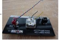
Now remove the insula4on completely from two 2cm pieces of the black wire, and solder one end of each piece of bare wire to the KEY pads on the main board. Be careful you don't catch your fingers on these when they are stuck up in the air!
