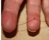
kink. Untwist the wire carefully. Trying to pull out the kink can snap the wire. Complete the 25 turns. They should occupy about three-quarters of the circumference. The 5 turn link winding, using red wire, is added over the centre of the main winding. Guess the centre, it is not really cri4cal
