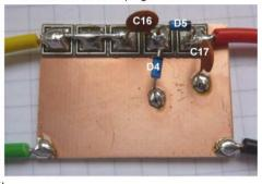
Tes4ng the transmier at this stage requires a Diode Probe. All the pa are provided for making such a probe a shown in the picture.
