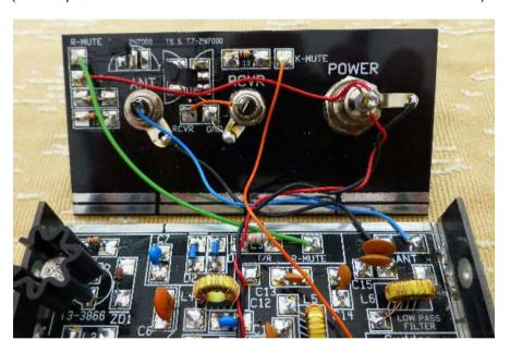
Finally, having finished the wiring to the back panel, you should solder the back panel in place using the same method that you used for the front panel. Be careful when soldering near the wires as the insula4on is easily damaged by the soldering iron. There is enough length to move them out of the way of the iron.
