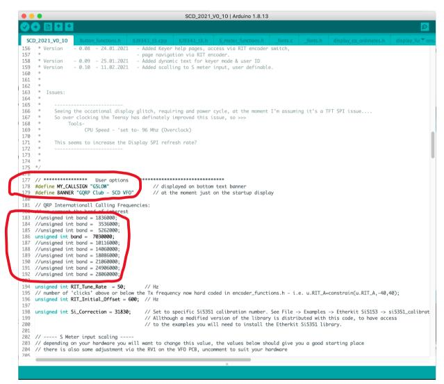
You can then reload the sketch and libraries by selecting the Teensy 3.2 and relevant COM port in the Arduino IDE.
