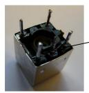
The oscillator coil, L3, is a 5u3L component, and the bandpass filter coils, L1 and L2, are 45u0L components.
