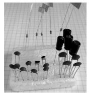
There is merit in following this order in construction. Note that the instructions refer to having the board so that the legends for the components read the correct way round (PP3 at the top right). The best results will come from the use of medium size soldering iron and Tin/Lead solder. It does help to set out all the components in the order they will be used. The best way is to use a small piece of polystyrene to hold the individual parts.
