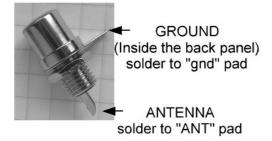
The antenna input socket is a single hole fixing 'phono socket'. It has a ground connection tag that needs to be inside the back panel. Bend this tag inwards for a wire that connects to the "gnd" pad. The antenna input connection is soldered to the "ANT" pad. Use differing colours to identify the two leads and twist them together.
