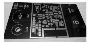
You will have noticed that this is a rather unusual kit. It has a printed circuit board without any holes. We call it "Limerick Construction" because it was designed by Rex Harper, W1REX, of Limerick, Maine. It is a surface mounted board in that the components are mounted on the surface of the board, although the components used
