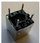
The oscillator coil, L3, is a 1u7H component, and the bandpass filter coils, L1 and L2, are 5u3L components.
