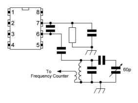
L3, the oscillator coil, has an unused link winding. This may be used to feed a frequency counter. Connect one (either) side of the link winding to ground and use the other end to connect to the counter. Some counters may detune the frequency a little so putting a low value capacitor (10 to 22pF) between the counter and the link winding is advised. Set the Tuning Capacitor control fully anti-clockwise and adjust the core to read
