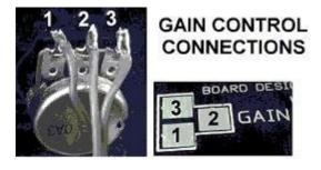
The gain potentiometer connections are shown; numbered 1, 2 and 3.
