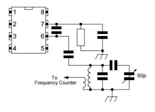
L3, the oscillator coil, has an unused link winding. This may be used to feed a frequency counter. Connect one (either) side of the link winding to ground and use the other end to connect to the counter. Some counters may detune the frequency a little so putting a low value capacitor (47 to 100pF) between the counter and the link winding is advised. Set the Tuning Capacitor control fully anti-clockwise and adjust the core to
