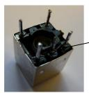
The oscillator coil, L3, is a 45u0L component, and the bandpass filter coils, L1 and L2, are also 45u0L components.
