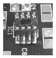
Tin the pads for IC1 and IC2.
