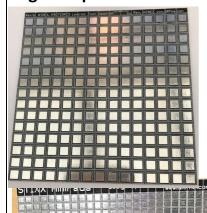
Rex has changed the size of these boards and they are now  $3\% \times 3\%$  (9.5 x 9.5cm) There are 225 squares in a 15 x 15 formation. The squares are % apart (6mm), and that includes a black solder mask. The board is routed on both sides so that the squares can be used in groups, or individually. The cost of these boards is £6.00 each, and postage is as for components.
