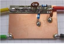
Tes5ng the transmier at this stage requires a Diode Probe. All the parts a provided for making such a probe as shown in the picture.
