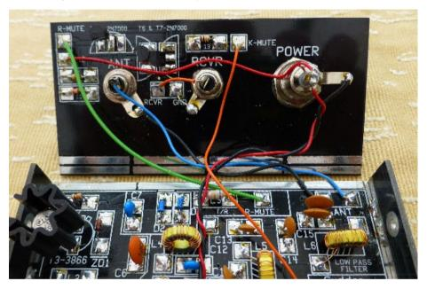
Finally, having finished the wiring to the back panel, you should solder the back panel in place using the same method that you used for the front panel. Be careful when soldering near the wires as the insula5on is easily damaged by the soldering iron. There is enough length to move them out of the way of the iron.
