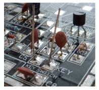
Now remove the insula5on completely from two 2cm pieces of the black wire, and solder one end of each piece of bare wire to the KEY pads on the main board. Be careful you don't catch your fingers on these when they are stuck up in the air!
