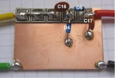
Tes2ng the transmier at this stage requires a Diode Probe. All the pa are provided for making such a probe a shown in the picture.
