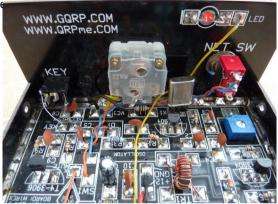
The layout of the printed circuit board. This shows the wirin**b**e-tween the pads
