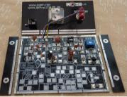
Like the side cheeks the front panel is soldered to the main board. This panel, unlike the side cheeks, overlaps the base board. The base board should be put in the gap between the soldered tracks at the boom of the front panel. This picture shows the correct posi2on of the front panel against the base. Again, we suggest that you use the "one blob" technique underneath the board to get the panel aligned correctly and ver2cal. Add a second blob when you are happy with the alignment.
