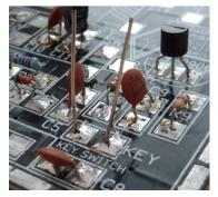
Now remove the insula2on completely from two 2cm pieces of the black wire, and solder one end of each piece of bare wire to the KEY pads on the main board. Be careful you don't catch your fingers on these when they are stuck up in the air!
