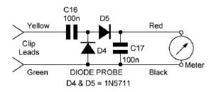
Yellow Clip Lead to top of R7 Green Clip Lead to ground Red lead with 4mm plug to Meter + Black lead with 4mm plug to Meter -
