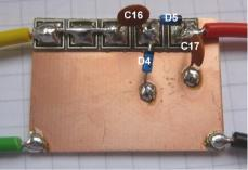
Tes4ng the transmier at this stage requires a Diode Probe. All the pa are provided for making such a probe a shown in the picture.
