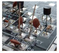
Now remove the insula4on completely from two 2cm pieces of the black wire, and solder one end of each piece of bare wire to the KEY pads on the main board. Be careful you don't catch your fingers on these when they are stuck up in the air! Add the side cheeks
