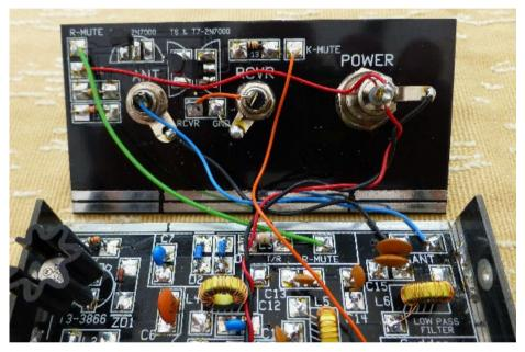
Finally, having finished the wiring to the back panel, you should solder the back panel in place using the same method that you used for the front panel. Be careful when soldering near the wires as the insula4on is easily damaged by the soldering iron. There is enough length to move them out of the way of the iron.
