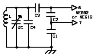
The circuit shows a typical Colpitts based VFO using an NE602 (or NE612) mixer.
