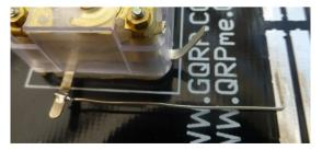
Next, using a short length of BT wire, connect the two bo\*om tag of the LOAD capacitor together and to the lower tag of S2, then connect the 470pF capacitor between the upper tag of S2 and the side ta the LOAD capacitor. For all these connec ons to the capacitor, make a small hook at the end of the wire, and squeeze it up to gently grip the capacitor tag.
