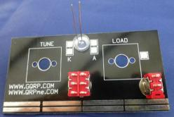
panel, the shorter lead is the kathode and is on the TUNE control side. Note the way up of the switch S2.
