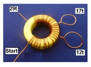
The Primary winding (shown above) has 29 turns of 20swg wire (the thickest wire), tapped at 12 turns and 17 turns. This requires about 50 inches of wire. Each pass of the wire
