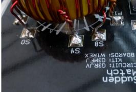
Finally for this stage of the construction, solder in the rest of the parts on the main board. It would be be\*er not to overheat the diode and make sure that you get it the right way round - both the diode and the board legend have polarity bars at the end. The resistors should be mounted, like the coil, by making a foot on the end of the wire thus having the resistors some 10mm above the board. This also applies to the ceramic capacitor.
