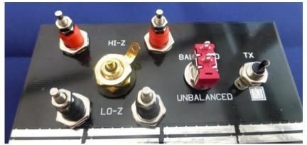
There is nothing awkward about moun ng most of these components - please make sure that the lipped insula ng washer that is part of the gold phono connector is fi\*ed into the hole properly from the socket side of the panel. This insulates the outer of the socket from the earthed PCB. You will need to bend the tag on the TX socket outer so it is easier to solder to.
